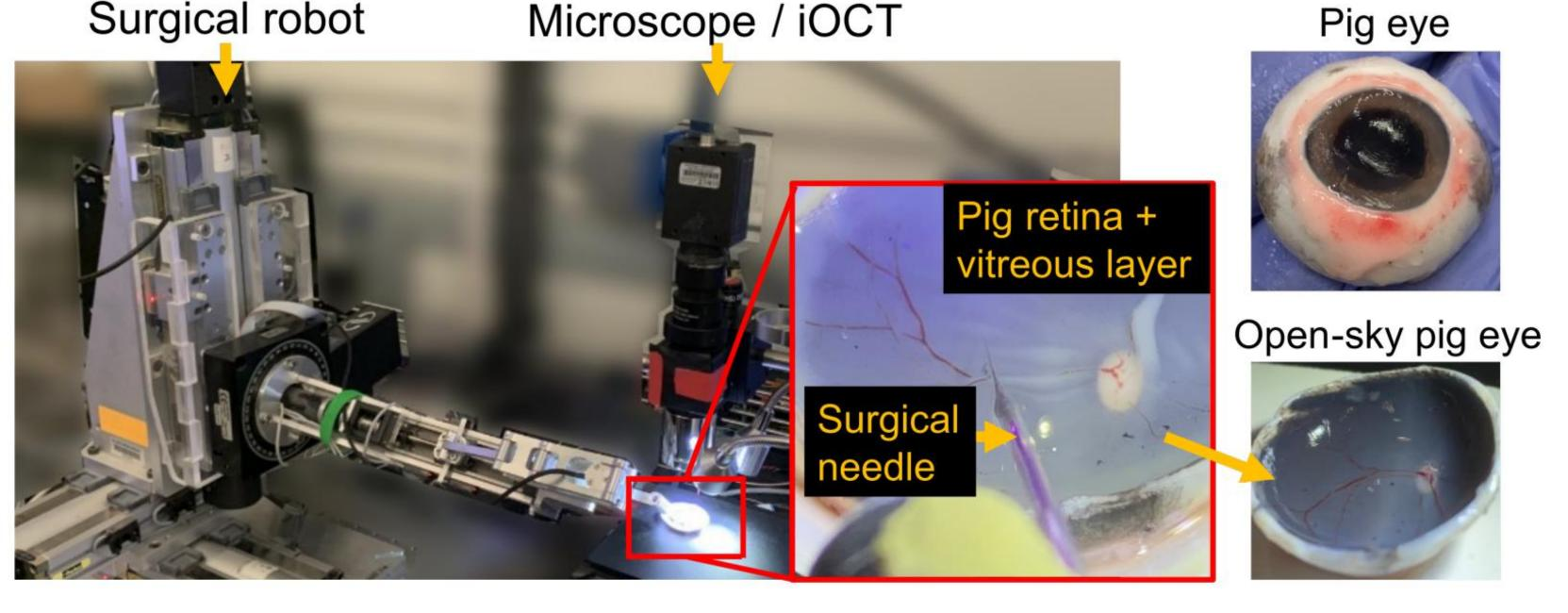
Our 5-dof robot arm enables precise motion, while the custom OCT-integrated microscope provides real-time RGB-D view for global and local awareness of the surgical environment
